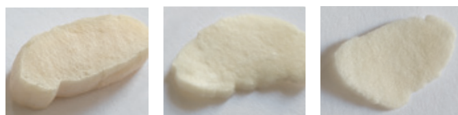
8 mm: Baypren® ALX 213-1 2 mm: Baypren® ALX 213-2 to 253-2 Baypren® ALX 310-1 to 340-1 1 mm: Baypren® ALX 340-2 to 350-2
